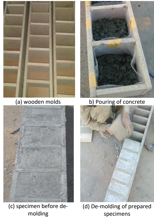
Figure 2 Preparation of concrete specimens
