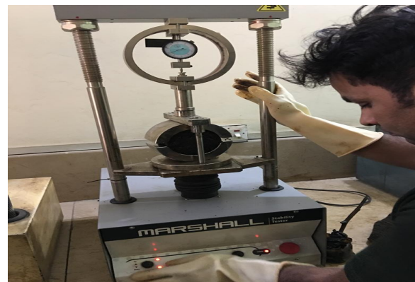
FIG 4. SAMPLE IN MARSHALL APPARATUS
