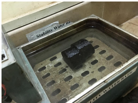
FIG 3. SAMPLES IN WATER BATH
