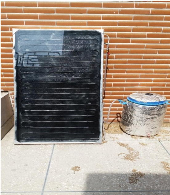
Figure 3. Fabricated flatbed solar water heater using cheap materials.
