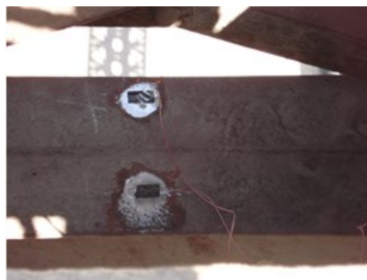
Figure 2 Strain gauges installed at different locations
