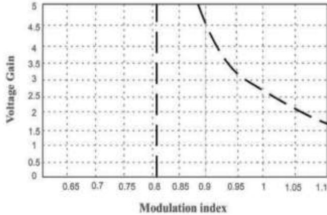
FIGURE 8. Voltage gain against MI with and without 3rd harmonic injection for max boost control
