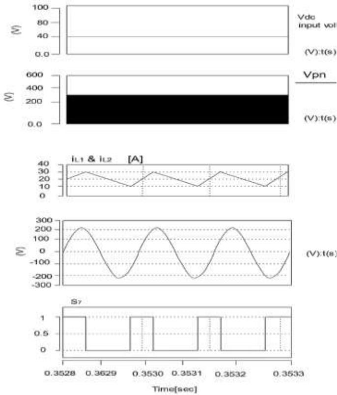
FIGURE 13. Simulation results for MBC
