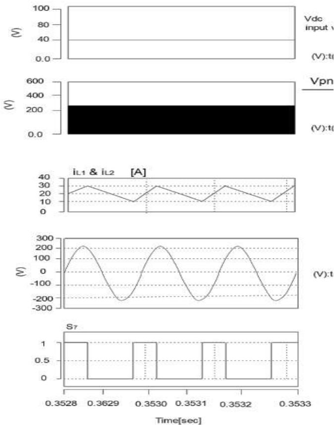
FIGURE 14. Simulation results of MBC with 3rd harmonic injection
