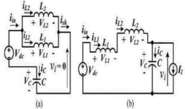
FIGURE 3. Equivalent circuits of ASC/SL-qZSI: (a) SH and (b) NSH
