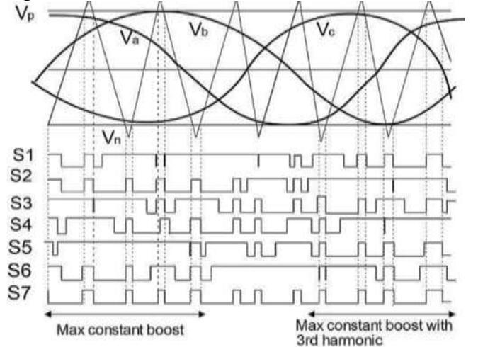
FIGURE 6. Switching scheme for max constant boost with and without 3rd harmonic injection
