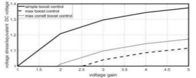
FIGURE 11. Stress ratio versus  $G$
