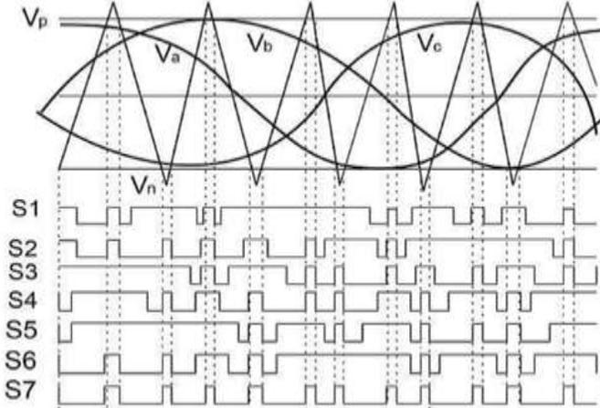
FIGURE 4. Switching Scheme for SBC
