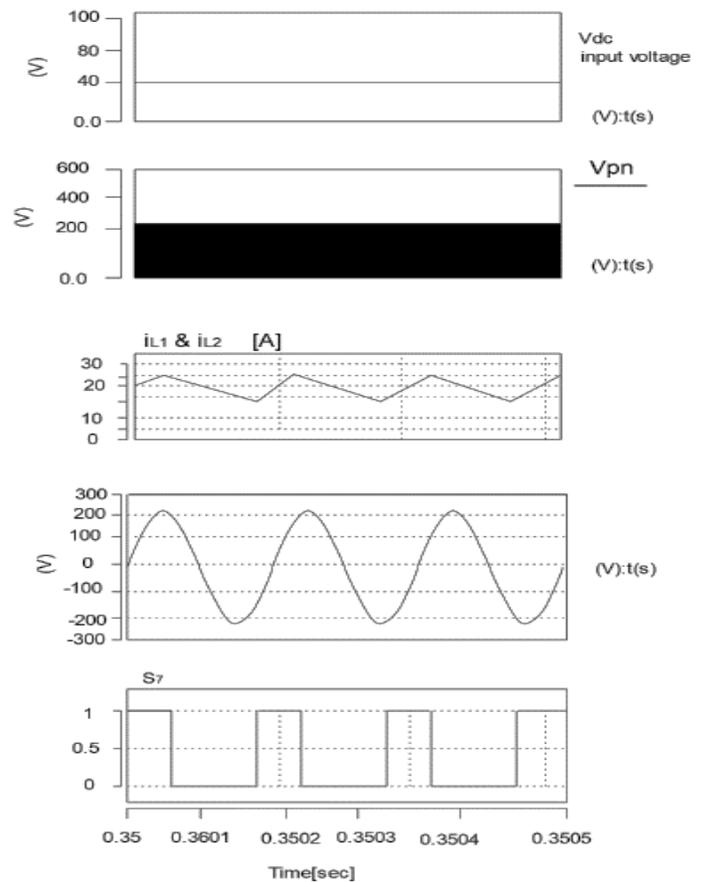
FIGURE 16. Simulation results for CBC with 3rd harmonic injection
