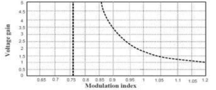
FIGURE 9. Voltage gain versus MI with 3rd harmonic injection for max boost control
