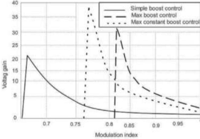
FIGURE 7. Voltage gain against MI
