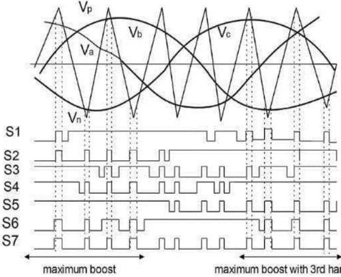
FIGURE 5. Switching scheme for max boost with and without 3rd harmonic injection
