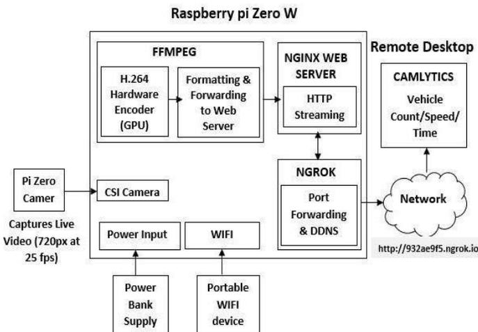
FIGURE 1. System Architecture of the proposed IoVT based solution
