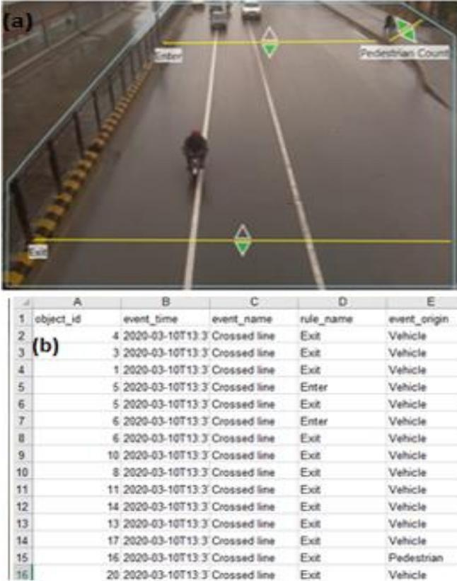
FIGURE 5 (a). Snapshot of streamed video in Camlytics installed on a Dell desktop. (b) Events generated during video analytics by Camlytics
