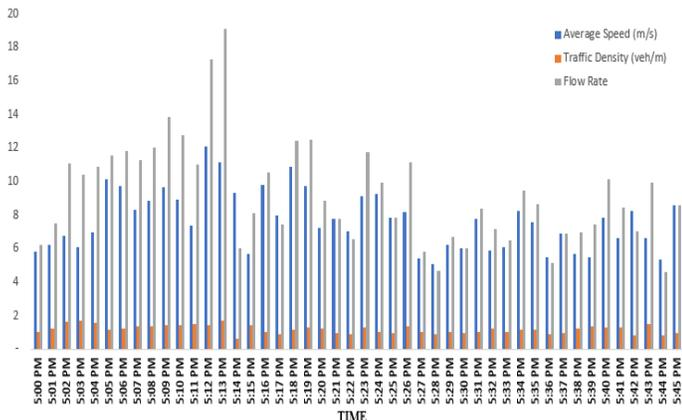
FIGURE 8. Traffic flow versus average speed versus road density on a 14m road section on Saturday, February 29th, 2022.
