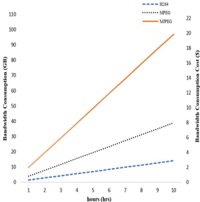
FIGURE 4. Data bandwidth requirement and cost per hour for live-streamed video using different Codec standards
