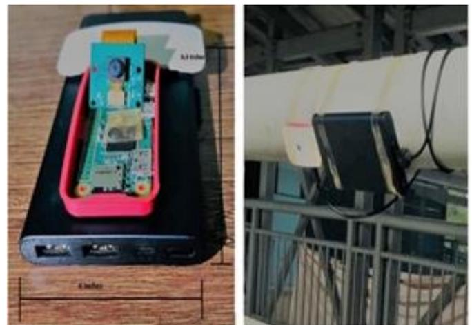
FIGURE 2. System hardware (a) Sensor Node (b) Sensor Node installed over the pedestrian bridge for evaluation
