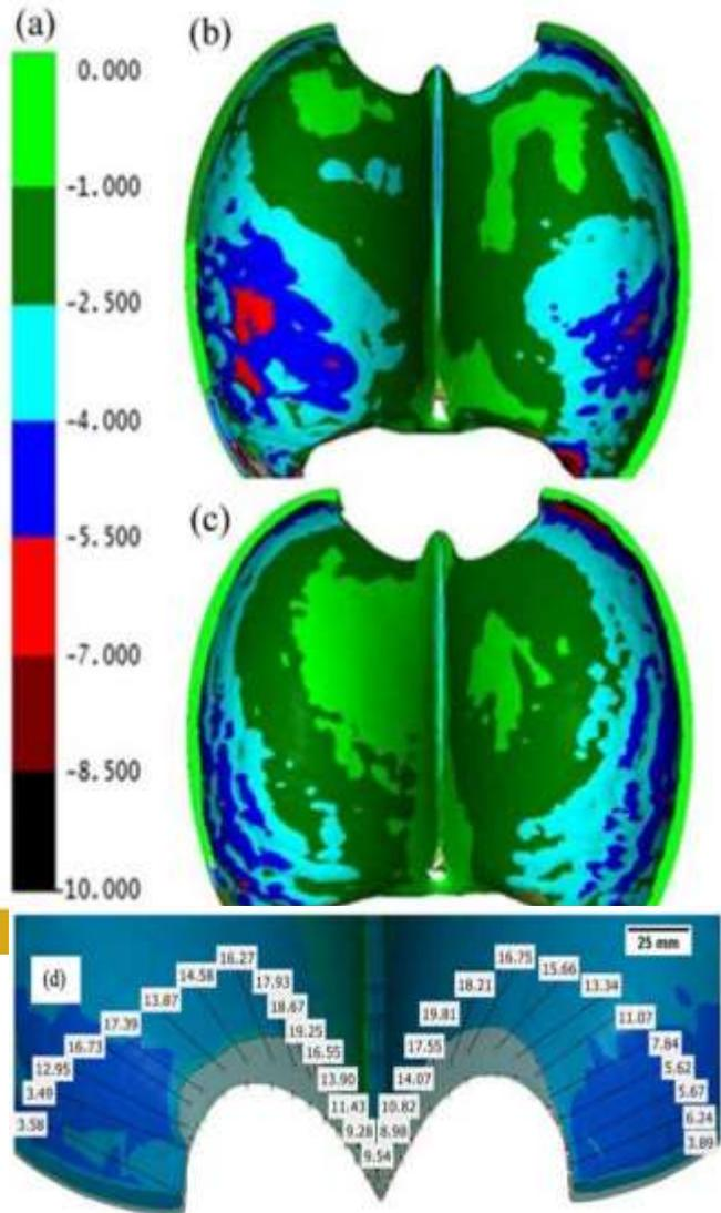
FIGURE 4. (a) Shows erosion depth in mm (b & c) Sediment erosion depth variation inside and outside the bucket (d) Erosion depth in cut-out region in mm [32]
