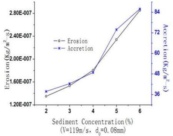
FIGURE 2. Erosion under different silt concentration [20].
