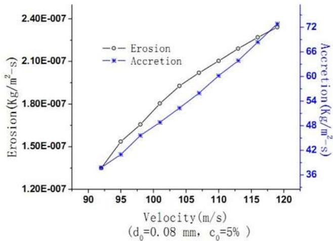
FIGURE 3. Influence of the Jet velocity on erosion [20].
