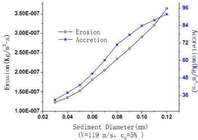
FIGURE 1. Erosion under different silt sizes [20].
