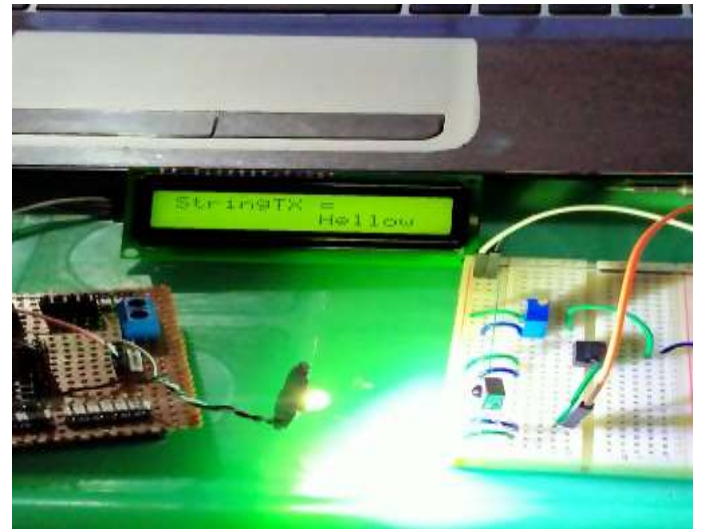
FIGURE 13. Testing Data "Hellow" on hardware.
