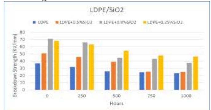
FIGURE 4. Change in Breakdown Strength (KV/mm) of LDPE/SiO<sub>2</sub> nanocomposites with aging
