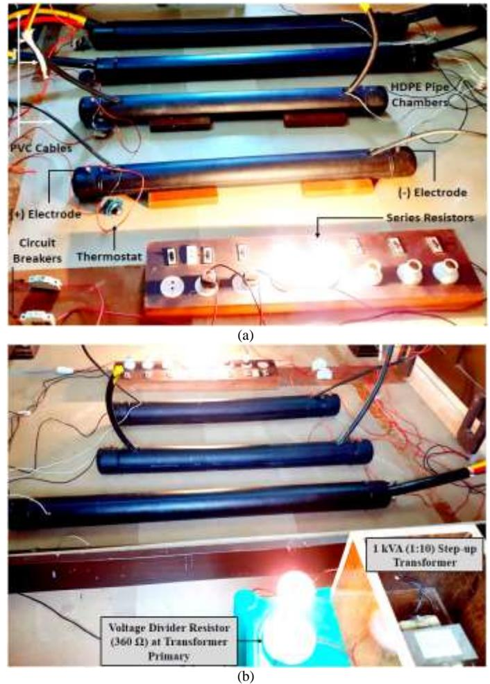
FIGURE 4. Experimental Setup of 1000 Hours Multistress Aging (a) Front View (b) Transformer Side View
