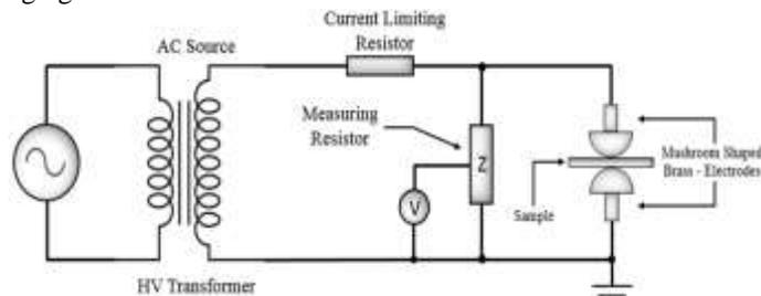
FIGURE 10. Schematic Diagram of Breakdown Test
