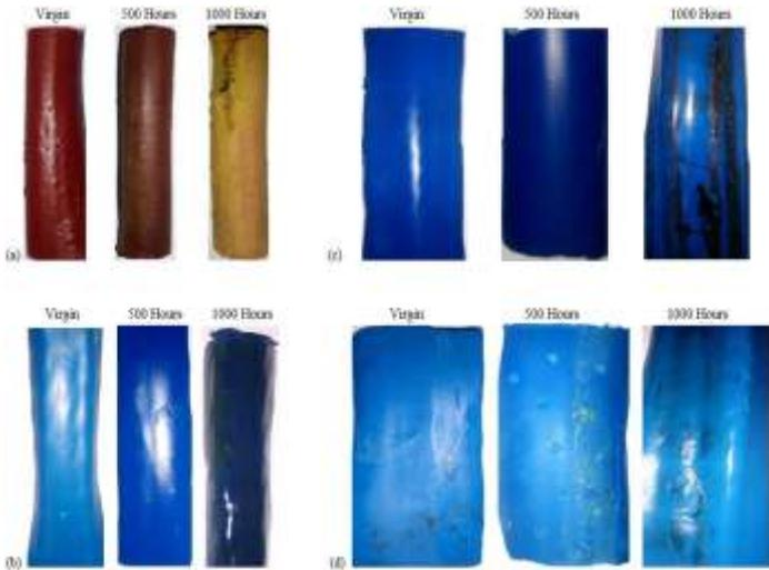
FIGURE 5. Insulation samples of virgin, 500 hours aged and 1000 hours aged PVC cables a) 2 core 10 mm<sup>2</sup>, b) 4 core 10 mm<sup>2</sup>, c) 4 core 120 mm<sup>2</sup> and d) 4 core 240 mm<sup>2</sup>
