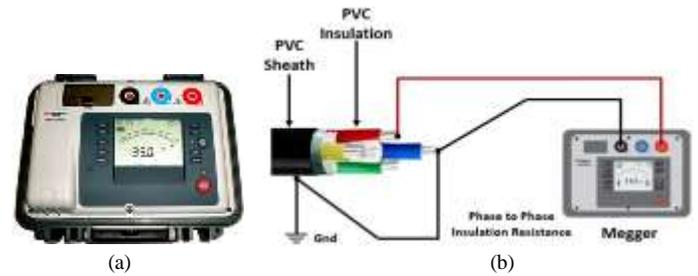
FIGURE 7. (a) Megger 10 kV (b) Insulation Resistance Test (Between Blue and Red cores phases)
