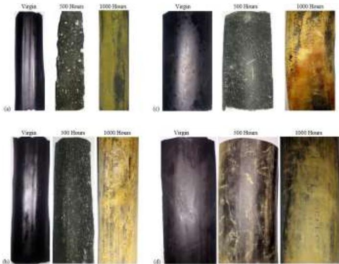
FIGURE 6. Sheath samples of virgin, 500 hours aged and 1000 hours aged PVC cables a) 2 core 10 mm<sup>2</sup>, b) 4 core 10 mm<sup>2</sup>, c) 4 core 120 mm<sup>2</sup> and d) 4 core 240 mm<sup>2</sup>
