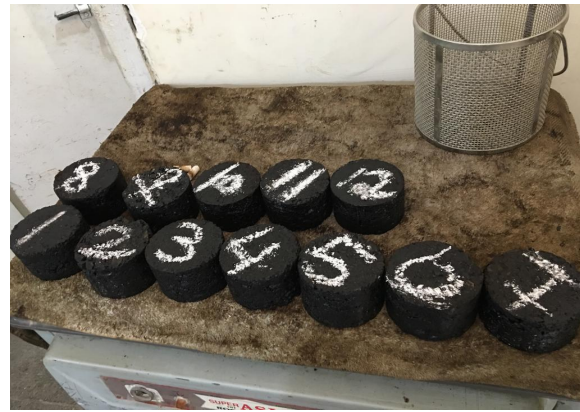
FIG 2. SAMPLES OF CS WITH ASPHALT MIX
