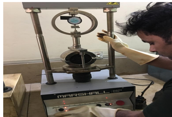
FIG 4. SAMPLE IN MARSHALL APPARATUS
